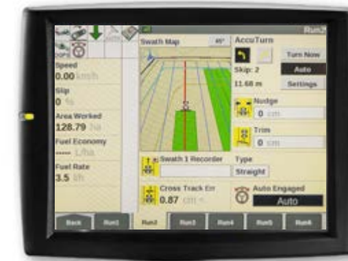
Automatizirani proces tokarenja s AFS AccuTurn Pro
